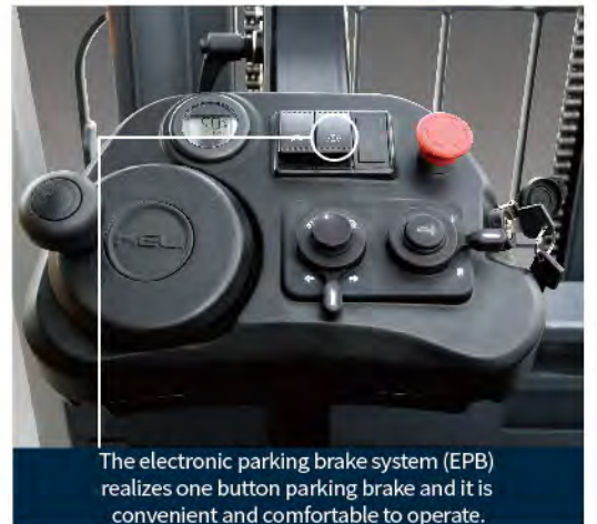
Rear handle with horn ensures stable driving posture when reversing and driving safety and comfort.
