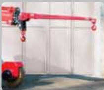
Optional searcher hook (Capacity: 150kg)
