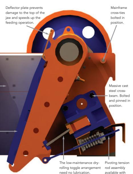
2 FULLY C Flywheels attached to shaft by Ringfeder shrink couplings. Stepless infinitely variable hydraulic adjusting system. Crusher setting can be adjusted at the touch of a button\* \*Auto-adjust is available
